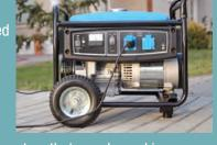
to backfeed— caused by generators that are plugged in or connected to a home's internal wiring. This is an extremely dangerous practice that presents an electrocution risk to utility workers and neighbors served by the same utility transformer. The only safe way to connect the generator to the house wiring is to have a licensed electrical contractor install a transfer switch in accordance with local electrical codes.
